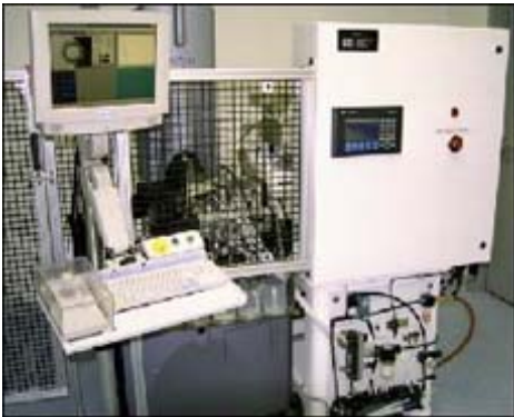
The time required to handle glass tubes and present them for inspection under a vision system is successfully reduced by a factor of 4.
